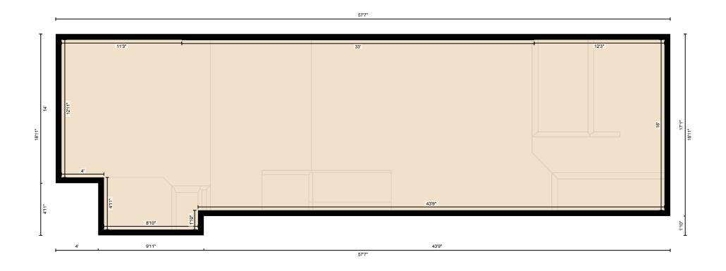
Measurement Diagram for: 2nd Floor Exterior Wall Thickness: 6.5 in
