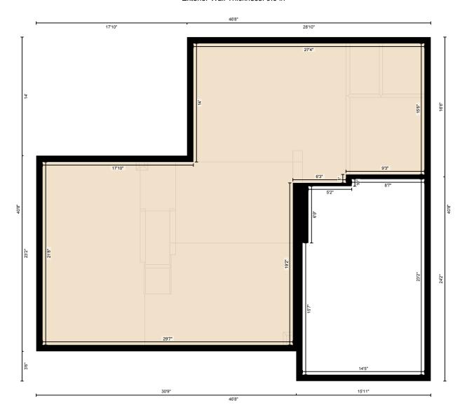
Measurement Diagram for: 1st Floor Exterior Wall Thickness: 9.0 in
