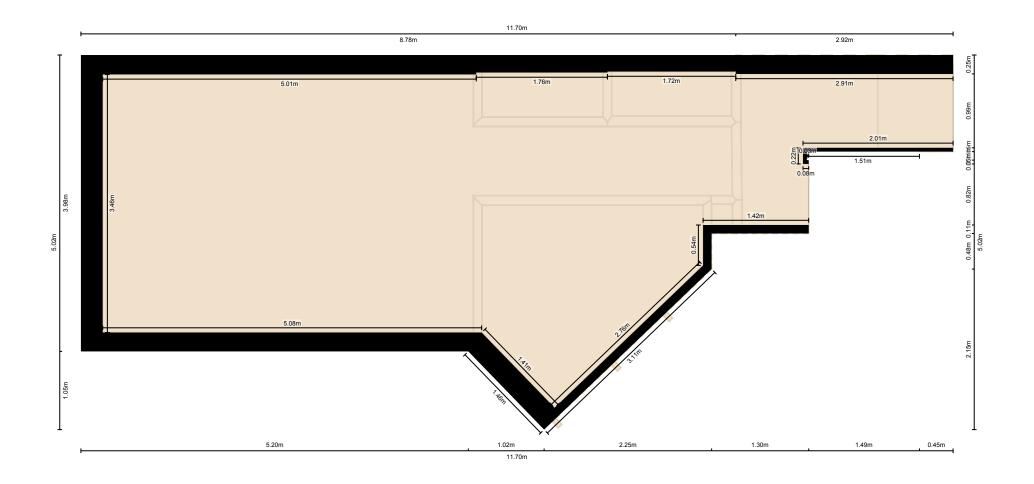
Measurement Diagram for: Top Floor Exterior Wall Thickness: 24 cm
