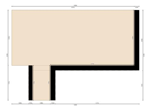
Measurement Diagram for: Basement Exterior Wall Thickness: 24 cm
