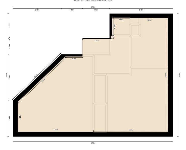
Measurement Diagram for: Lower Den Exterior Wall Thickness: 24 cm
