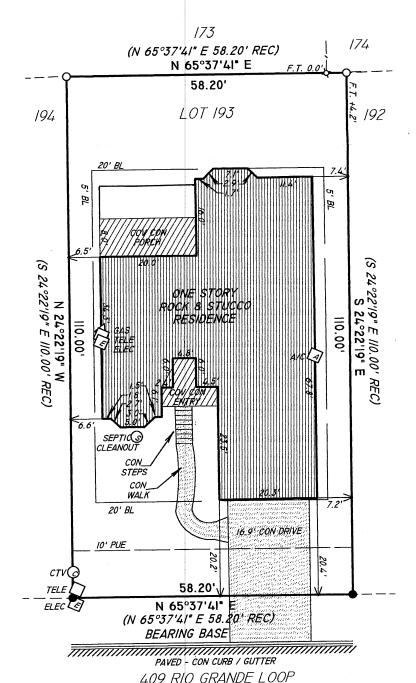
BUILDING SETBACKS 20' FRONT - V/80-86 20' REAR - V/80-86 5' SIDE - V/80-86 EASEMENTS 10' FRONT - V/80-86
