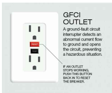
GFCI plug receptical
