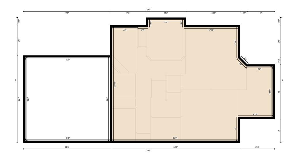
Measurement Diagram for: 2nd Floor Exterior Wall Thickness: 6.5 in
