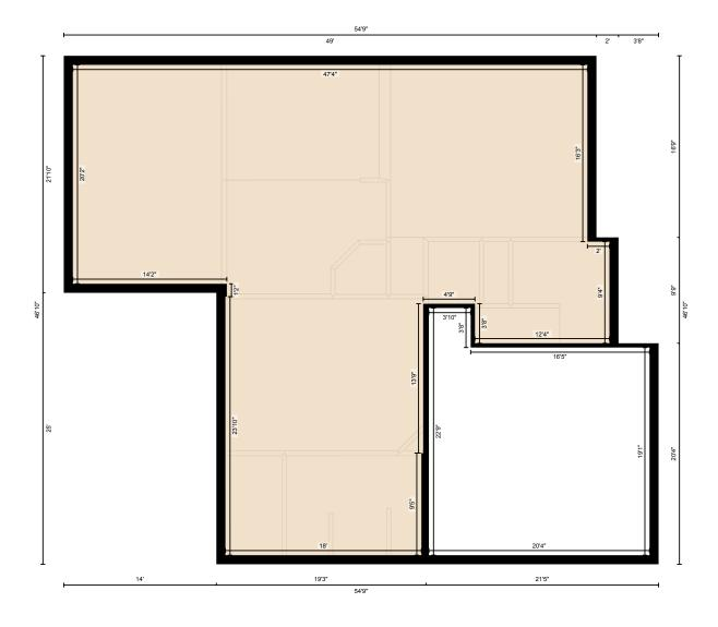
Measurement Diagram for: 2nd Floor Exterior Wall Thickness: 10.0 in
