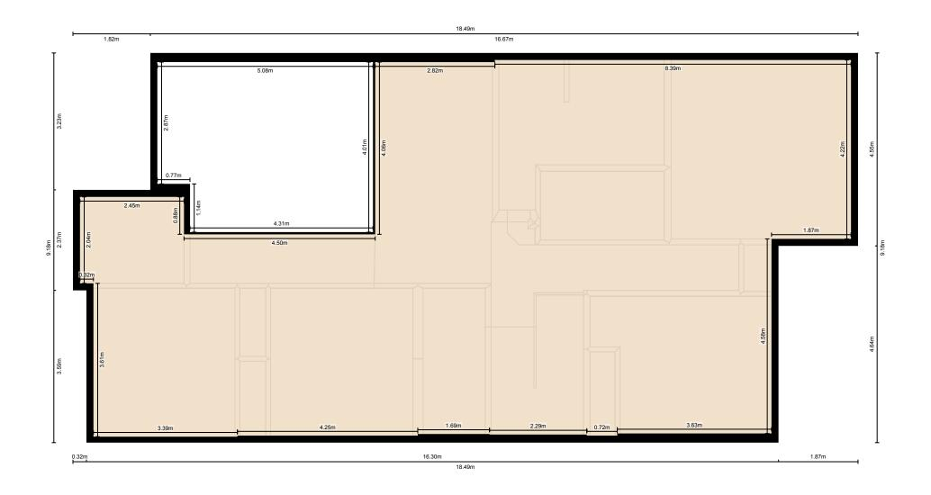
Measurement Diagram for: Basement Exterior Wall Thickness: 17 cm
