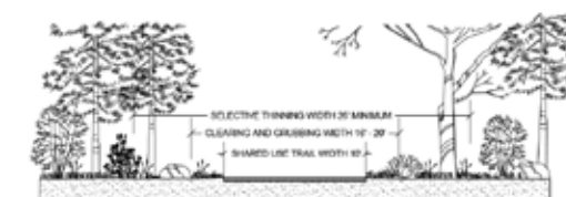
TYPICAL SHARED USE PATH SECTION
