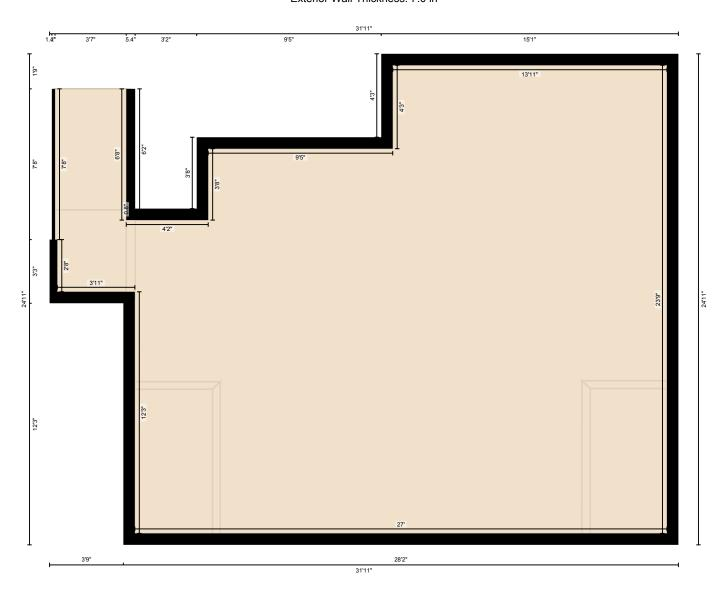
Measurement Diagram for: Basement Exterior Wall Thickness: 7.0 in
