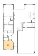
Max Dimensions: 13'1" x 12'10" Calculated Area: 147 sq. ft Included: Yes Heated: Yes Finished: Yes Enclosed: Yes Contiguous: Yes Permitted: Yes Wet space: No Addition: No Conversion: No
