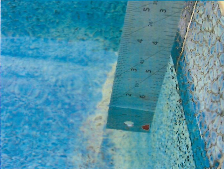
12. Water level at northeast corner measures 6-1/2" below top of coping.
