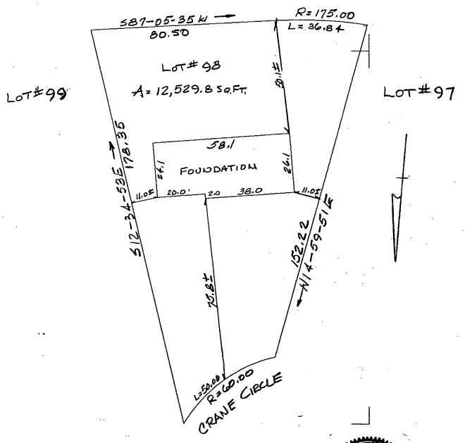
I HEREBY CERTIFY TO ROBO DEVELOPMENT CORP. THAT THE FOUNDATION ON THIS LOT IS LOCATED AS SHOWN, I FURTHER CERTIFY THAT IT CONFORMS TO THE ZONING LAWS OF THE TOWN OF SHREWSBURY WITH RESPECT TO DIMENSIONAL SETBACK AND IT DOES NOT LIE WITHIN AN ESTABLISHED FLOOD HAZARD ZONE. THIS CERTIFICATION IS NON—TRANSFERABLE.
