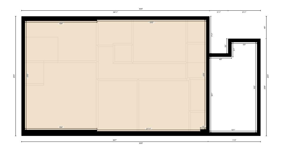
Measurement Diagram for: 2nd Floor Exterior Wall Thickness: 9.1 in
