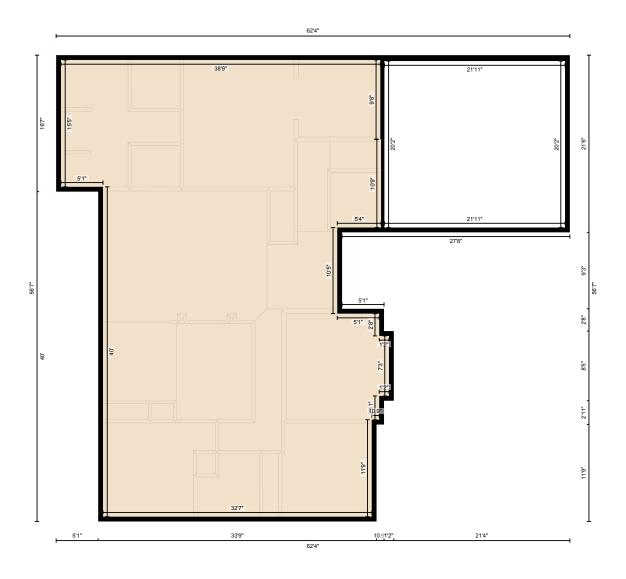
Measurement Diagram for: Bonus Room Exterior Wall Thickness: 7.0 in
