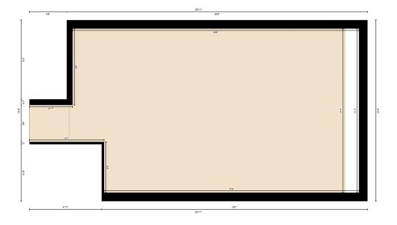
Measurement Diagram for: Garage Lower Level Exterior Wall Thickness: 7.0 in
