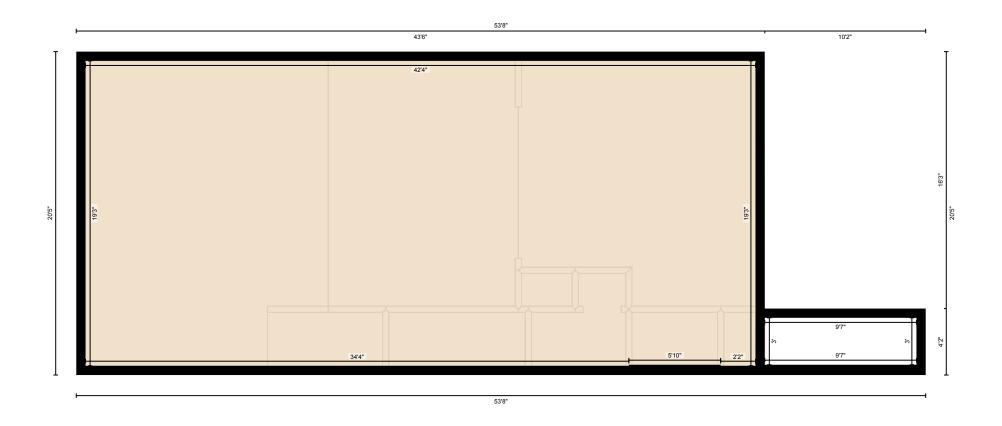
Measurement Diagram for: 2nd Floor Exterior Wall Thickness: 7.0 in
