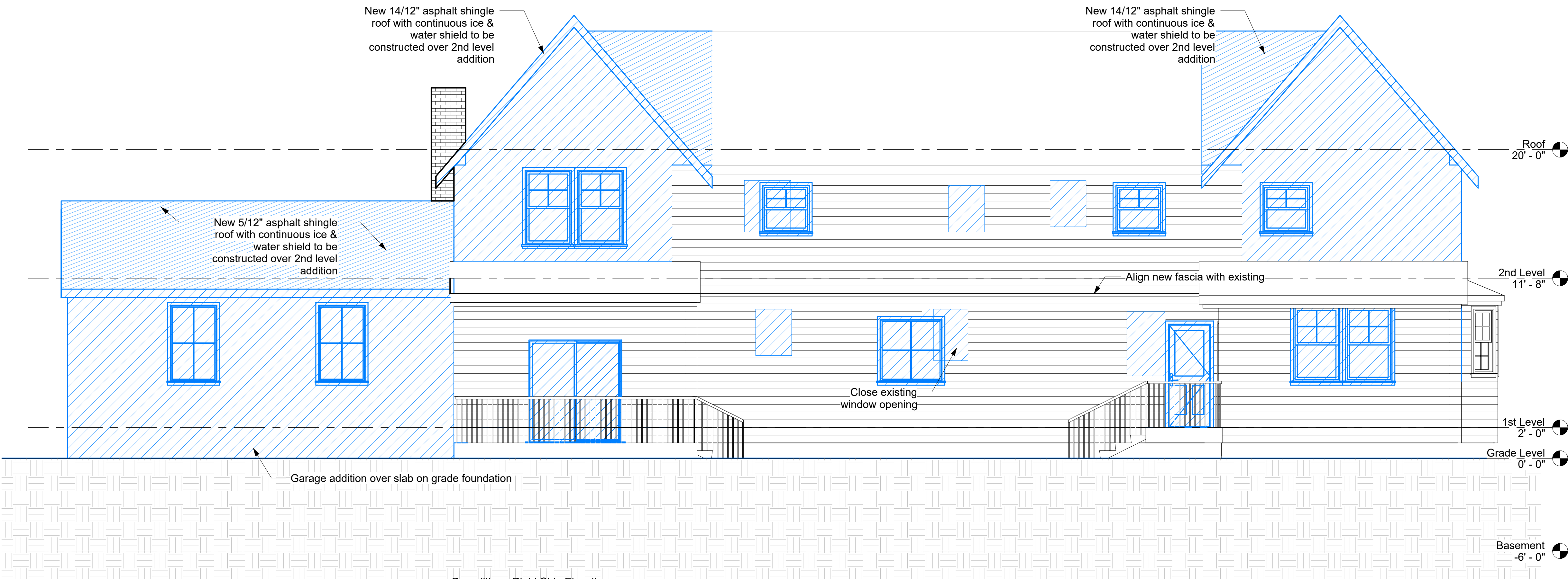
② Demolition - Right Side Elevation 1/4" = 1'-0"
