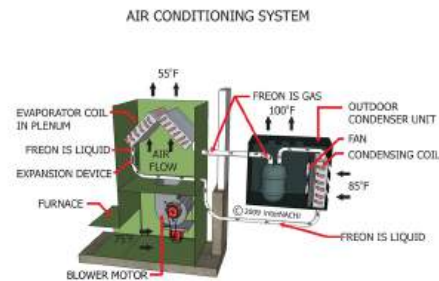
air conditioning system
