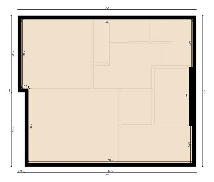
Measurement Diagram for: 3rd Floor Exterior Wall Thickness: 17 cm
